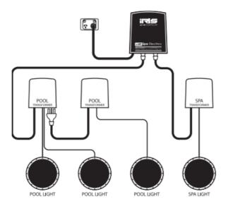
Note: For systems with 2 or more pool lights, use the LV50-12 transformer andutilise the piggyback feature on the LV50-12 to ensure all transformers are switched together.
