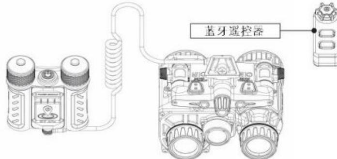
When using, please open the J-FB battery compartment and connect the cable to the J-FB night vision device before turning on infrared mode. At the same time, press the J-FB Bluetooth remote control button to wake up from sleep, and then operate the J-FB host to enter the corresponding Bluetooth settings in the menu to complete the connection of the Bluetooth remote control.
