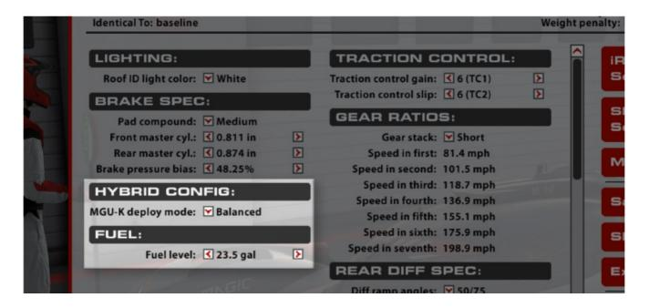
The Acura ARX-06's hybrid system can be set to one of five deploy modes to alter the target State of Charge (SoC) for the end of a lap. Each of these modes will use varying levels of energy throughout a lap to reach a target, and thus some will produce more power over the course of a lap and faster lap times at the cost of discharging the battery.
