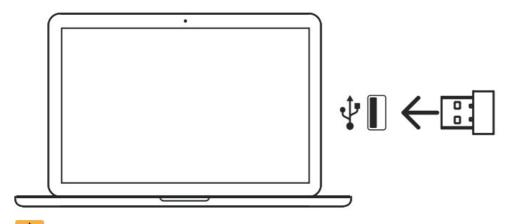
3. Press to enter 2464z connecting mode. The indicator turns off when the keyboard is connected successfully.
