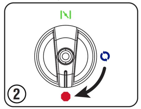
3. Turn the fuel cap vent lever to the "OFF" position.
