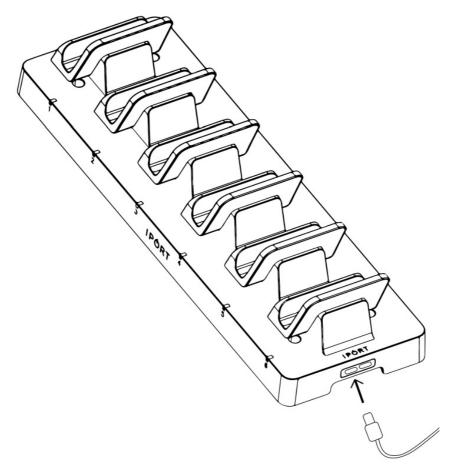
4. Additionally, use the second USB-C Port to plug in a second 72309 to link the two together. You can link up to 3 additional MultiDocks.
