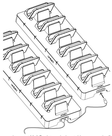
5. Optional – to securely mount MulitDock to a desk or table, remove the first and last charging cradles (see step 6), insert the provided screws through thefour openings on the MultiDock and hand tighten with a screwdriver.
