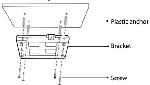
• **Option B:** Align the plastic nuts with the holes in the ceiling, and use the included screws to fix the bracket.
