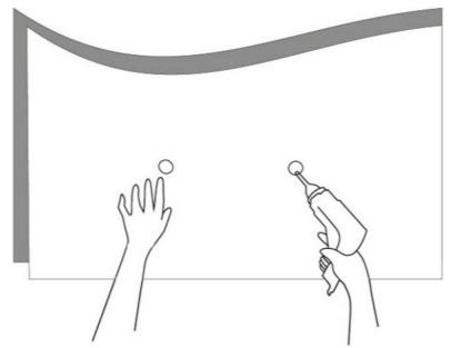
3. Knock the plastic anchors into the holes using the rubber hammer. Then use the screwdriver to tighten the screws into the plastic anchors.
