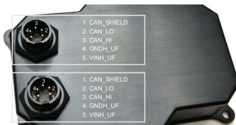
Figure 3 - Connector Pinout
