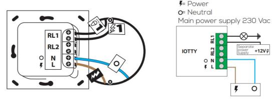
Electrical scheme for a load that needs a pulse to activate:
