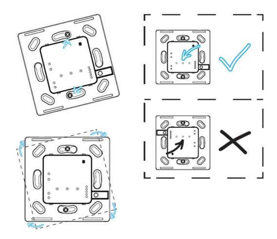
Push all the wires back into the wall box (do not push the wires using the back of the switch). Insert the device in the wall box and screw it in. Position the switch so that the AP and reset buttons are located on the left.
