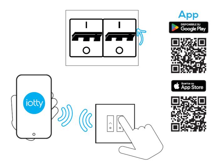
Turn on the power at the circuit breaker. Check if the wiring was made correctly by tapping on the glass to activate the shade. Now the installation is complete and you can proceed to register the device.
