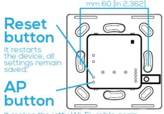
It makes the iotty Wi-Fi visible again. Useful to re-register the device on the app, update the Wi-Fi credentials, or turn off the device Wi-Fi.
