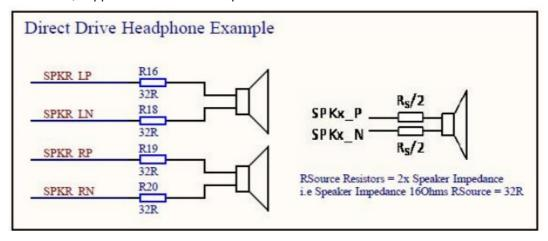
To achieve optimal audio performance in direct drive applications the DACs should operate at close the maximum output voltage of 1Vrms. This can be achieved by adding source resistors between the output terminals and the speaker driver, the value of which are double the rated speaker impedance. i.e., for  $16\Omega$  speakers use  $32\Omega$  resistors, for  $32\Omega$  speakers use  $64\Omega$  resistors.
