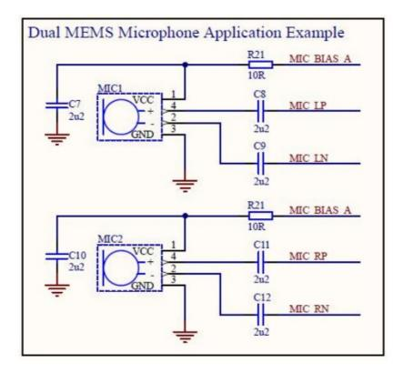
If a single microphone is used, the unused analogue inputs should be AC coupled to ground.
