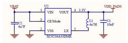
To save the cost of an external regulator the VDD\_PADS input can be connected direct to the battery input as long as all digital peripherals are tolerant of the variation of the battery voltage over its entire operating range of 2.8V to 4.24V (VFloatmax).
