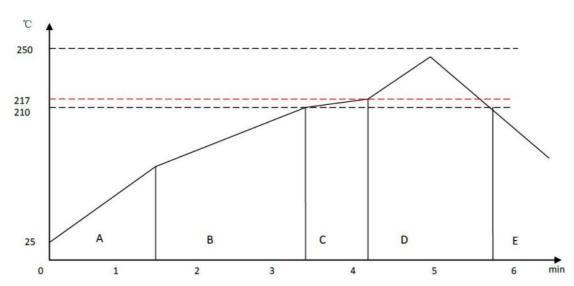
Zone A: Preheat: This raises the temperature at a controlled rate, typically 0.5 - 2C/s. This will preheat the component to  $120^{\circ}$ C to  $150^{\circ}$ C to distribute the heat uniformly to the PCB.
