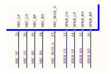
All analogue inputs are DC coupled and must be externally ac coupled for correct operation. Stereo Line In
