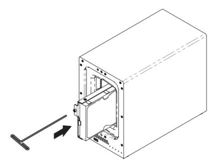
6. Replace the waterproof drive cover and securely tighten it using the 3mm hex tool.
