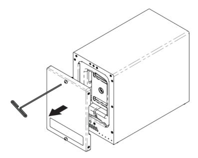
2. Remove the waterproof drive cover with the 3mm hex tool.
