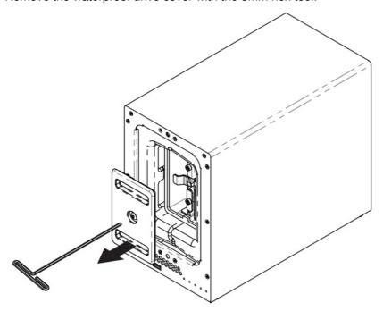
3. Remove the drive trays with the 3mm hex tool.
