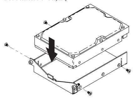
5. Insert each loaded drive tray into an empty drive bay, ensuring that each one is pushed in all the way. Then tighten the screws using the 3mm hex tool.
