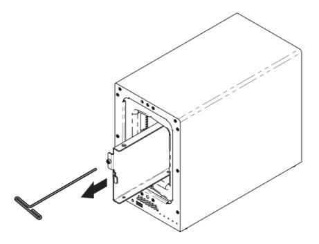
4. Install a compatible drive into each drive tray using (4x) drive screws and a Phillips screwdriver. Visit <a href="iosafe.com/support/hardware-compatibility">iosafe.com/support/hardware-compatibility</a> for a list of qualified drive models.
