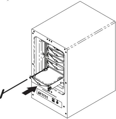
f. Replace the waterproof drive cover and securely tighten it using the 3mm hex tool. **STOP** Avoid using tools other than the supplied hex tool to secure the waterproof drive cover as you could undertighten or break the screw. The hex tool has been designed to flex slightly when the screw is sufficiently tight and the waterproof gasket is properly compressed.
