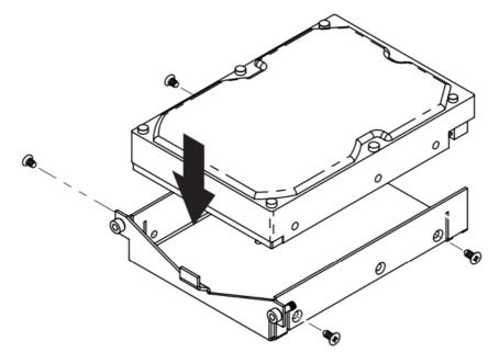
e. Insert each loaded drive tray into an empty drive bay, ensuring that each one is pushed in all the way. Then tighten the screws using the 3mm hex tool.
