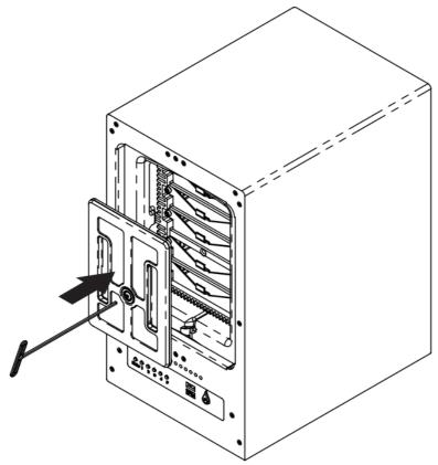
g. Install the front cover to finish the installation and protect the drives from fire.
