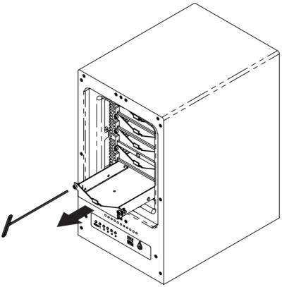
d. Install a compatible drive into each drive tray using (4x) drive screws and a Phillips screwdriver. Please visit iosafe.com for a list of qualified drive models.
