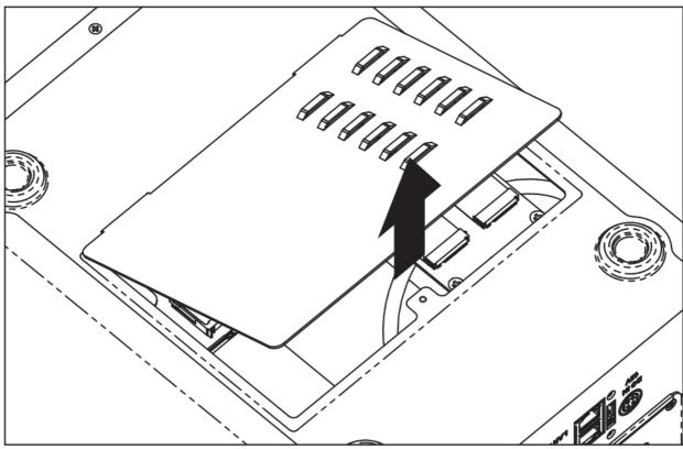
d. Remove the plastic retainer clip from the rear of the SSD slot(s) you intend to use.
