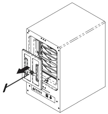
c. Remove the drive trays with the 3mm hex tool.
