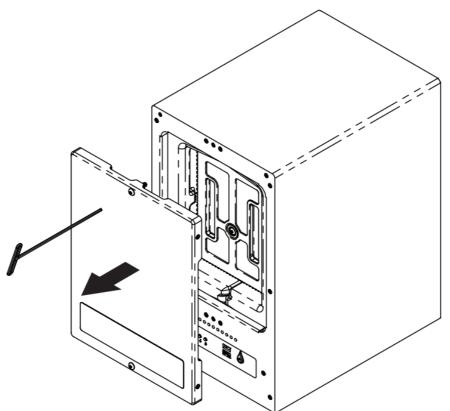
b. Remove the waterproof drive cover with the 3mm hex tool.
