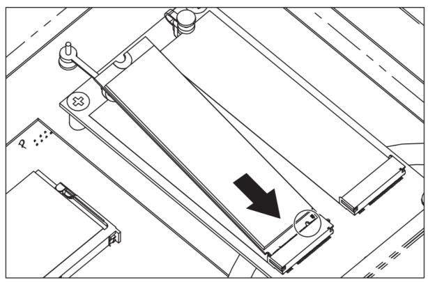
f. Hold the SSD module flat against the slot bay (Fig. 1) and reinsert the plastic retainer clip back into the rear of the slot to secure the SSD module. Press down firmly to secure the clip in place (Fig. 2).
