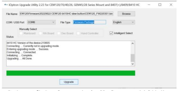
4. Power cycling the mount. Check your firmware version after all four firmware upgrade is finished by press MENU Firmware Information.
