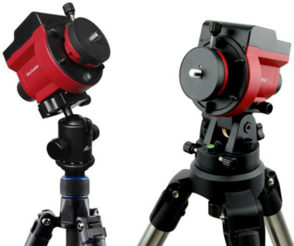
To use the alt-azi base, just simply slide the mount head base into the alt-azi base dovetail saddle. You can slide the mount head in from either direction depending on your latitude position and payload. The latitude adjustment range can be from  $-30^{\circ}$  to  $65^{\circ}$ . If possible, choose the one with the center of gravity of the system as close to the center of the base as possible.
