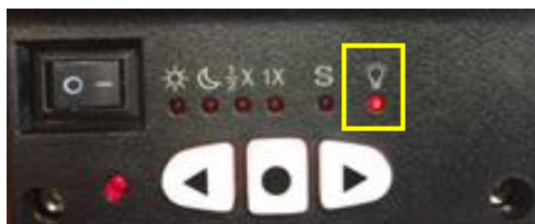
When done light intensity adjustment, double-check the LED under letter "S" to make sure the correct
