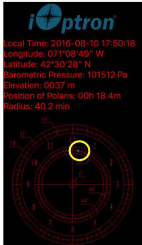
Press the power switch on the mount to turn on the mount. Look through the polar scope eyepiece. If you can not see red polar scope dial or a large tick mark is not on top, release RA Clutch Disk slightly. Rotate the RA axis until you see the red LED illumination and/or adjust one of the large tick mark to the top. Lock the RA axis again. Adjust the eyepiece to bring the reticle dial in focus.
