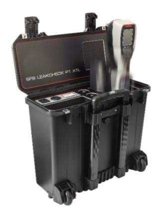
Wait for any action until working position. Take one P1 SmartSensor out of the storage bay.
