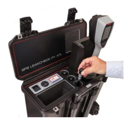
Attach the P1 SmartSensor into the plug at the handgun before you switch the instrument on.
