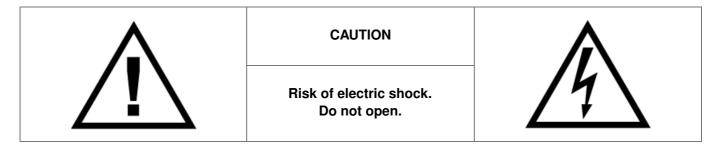
**DANGEROUS VOLTAGE:** The lightning flash with arrowhead symbol within the equilateral triangle is intended to alert the user to the presence of un-insulated "dangerous voltage" within the product's enclosure that may be of sufficient magnitude to constitute a risk of electric shock.
