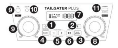
1. Power Button: Turns Tailgater Plus on or off. Please note that while Tailgater Plus is connected to a power
