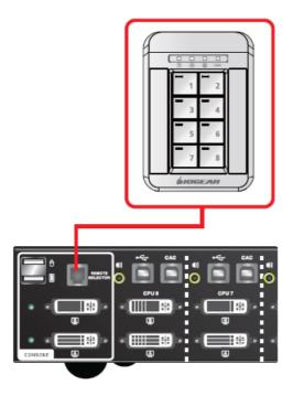
**Warning** – If a mechanical intrusion is detected by the RPS (connected with the switch and aligned), this will permanently disable both the RPS itself and the switch and all LEDs (on RPS) and the front panel LEDs except the Power LED (on switch) will flash continuously.
