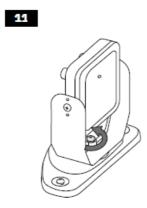
Note: to avoid damaging the bracket, loosen the screw completely before panning the sensor.
