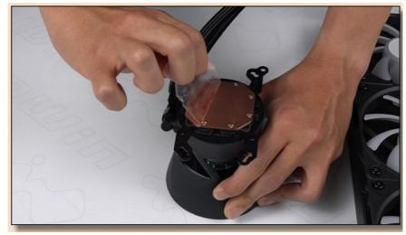
• D. Install the water block and then tighten it with the Thumbscrews.
