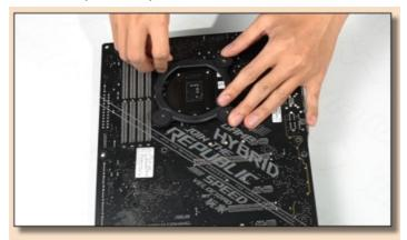
3. Install the standoff screws onto your motherboard. Ensure to use the correct standoff screws for your CPU socket.
