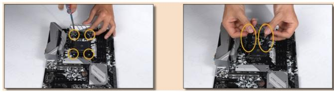
2. Install the standoff screws onto your motherboard. Ensure to use the correct standoff screws for your CPU socket. Parts Required: Standoff Screws (AMD or TR4)
