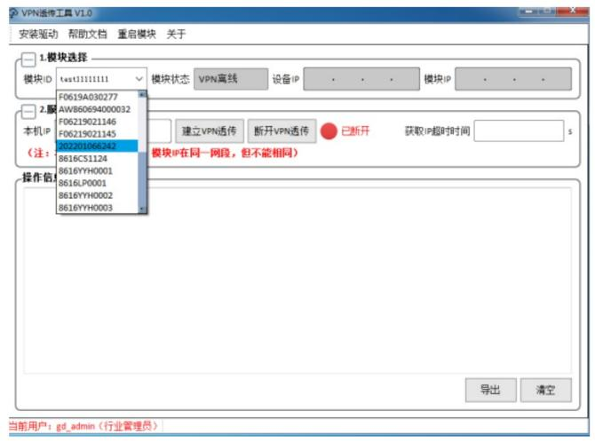
5. After the module ID is selected, the information of the module (including module ID and device VPN online state) will be displayed automatically. Module VPN offline indicates the current module does not use the VFD pass-through function. Module VPN online indicates the current module is performing pass-through and cannot
