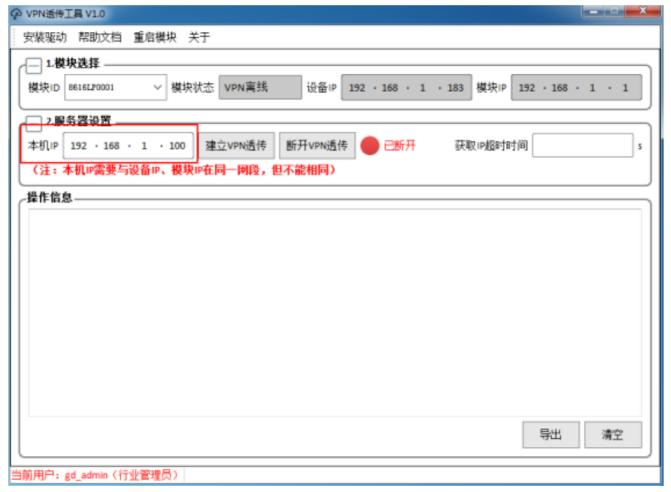
7. After the setting is complete, click Establish VPN pass-through, and the connection process will take one to two minutes. When "The configuration is complete, and VFD pass-through is performing" is displayed, it indicates that VPN channel is established successfully and VFD pass-through can be conducted. If you need to exit the VPN passthrough, you can click Disconnect VPN pass-through.
