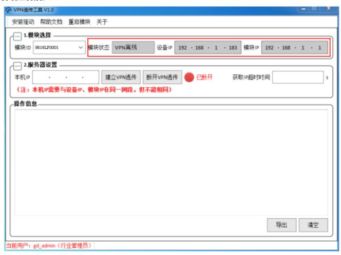
6. Set the local virtual IP. Note that the local IP needs to be in the same network segment with the device IP and module IP of the PLC/VFD but they cannot be the same. Obtain IP timeout time is null by default, and you have no need to set it. Device IP can be set in the module strategy file, which is consistent with IP of the VFD/PLC
