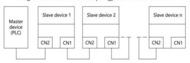
Figure 2-4 Star network topology electrical connection
