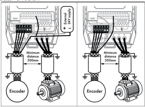
Alternatively (to External supply) the drives on-board 24V supply can be used (T1 (24V) and T7 (0V)) – Ensure total current consumption from T1 does not exceed 100mA.
