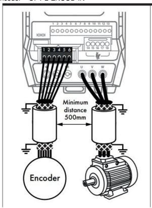
**NOTE** Do not connect the encoder cable shield to OV of the drive or encoder module.
