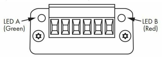
The fault code is indicated on the drive display. Please see Error Code Defi nitions. For transient faults, the LED will remain illuminated for 50ms to notify a fault on the module.
