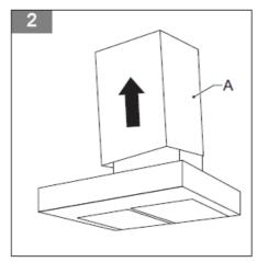
2. Remove the shaft (A) of the extractor hood (extraction) or remove the carbon filter (recirculation).
