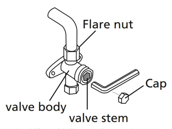
Using hexagonal wrench, fully open both the high pressure and low pressure valves.
