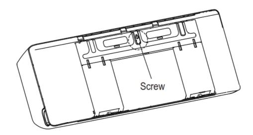
• Secure the mounting plate to the wall with the screws provided. Make sure that mounting plate is fiat against the wall.
