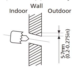
**NOTE:** When the gas side connective pipe is  $\Phi$  16mm(5/8in) or more, the wall hole should be 90mm(3.54in).
