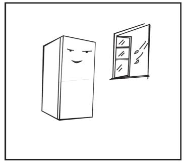
• The refrigerator is placed in a well-ventilated indoor place; the ground shall be flat, and sturdy (rotate left or right to adjust the wheel for leveling if unstable).
