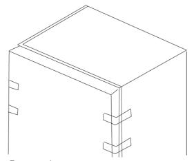
3. Unscrew screws of the top cover, Remove the top cover.
