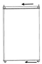
8. Put down the door on bottom hinge vertically. Fix the upper hinge, fix top cover of refrigerator.
