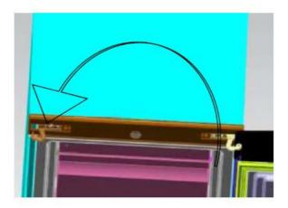
8. Set the top door right position, fix the top hinge and the cover
