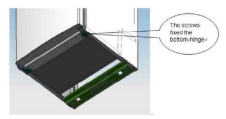
5. Replace the bottom hinge to the other side then fix It with screws.
