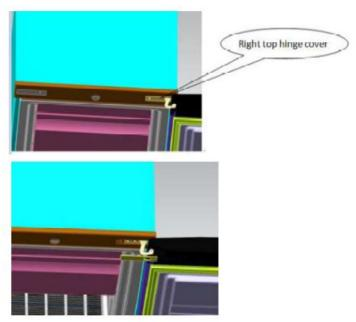
2. Remove the screws fixing the top hinge with a cross-slot screwdriver.
