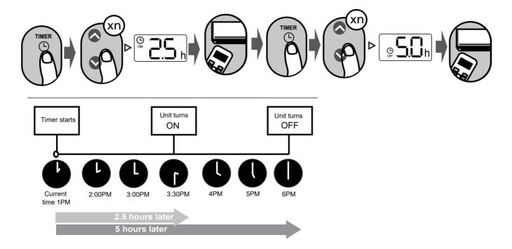
**Example:** If the current timer is 1:00 PM, to set the timer as the above steps, the unit will turn on 2.5h later (3:30 PM) and turn off at 6:00 PM.
