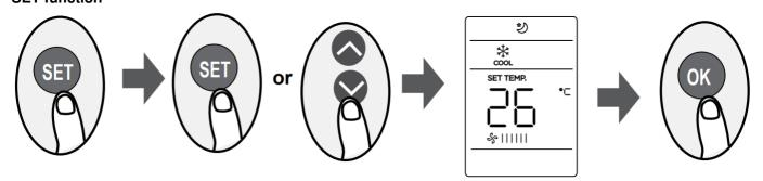
Press the SET button to enter the function setting, then press the SET button or TEMP  $\land$  or  $\lor$  TEMP button to select the desired function. The selected symbol will flash on the display area, press the OK button to confirm. To cancel the selected function, just perform the same procedures as above.
