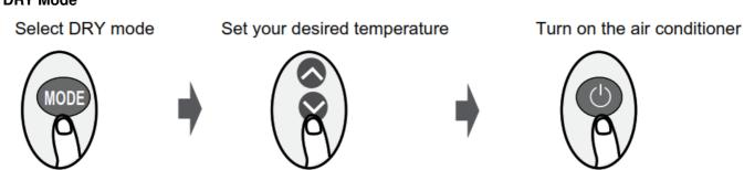
**NOTE:** In DRY mode, fan speed can not be set since it has already been automatically controlled. **FAN Mode**
