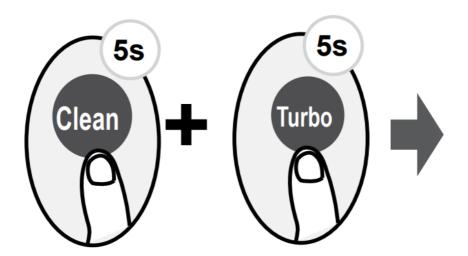
Press together the Clean button and Turbo button at the same time for more than 5 seconds to activate the Lock function. All buttons will not respond except pressing these two buttons for two seconds again to disable locking. **SET function**
