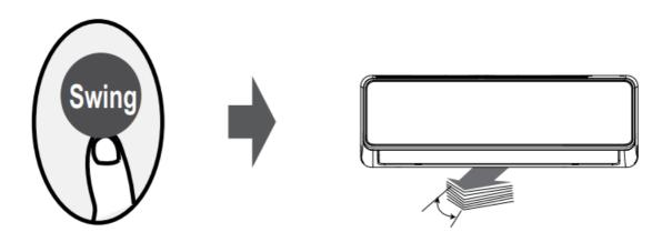
The horizontal louver will swing up and down automatically when pressing Swing button. Press again to make it stop.
