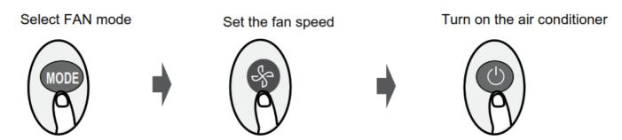
**NOTE:** In FAN mode, you can't set the temperature. As a result, no temperature displays in the remote screen.
