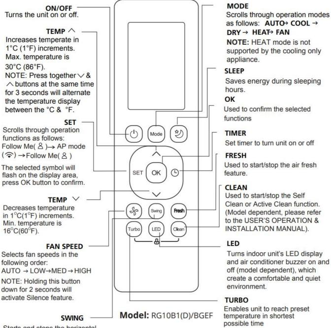
Starts and stops the horizontal louver movement. Hold down for 2 seconds to initiate vertical louver auto swing feature.
