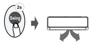
Keep pressing this button more than 2 seconds, the vertical louver swing function is activated. (Model dependent)
