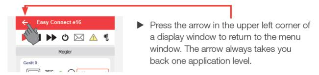
• Press the arrow in the upper left corner of a display window to return to the menu window. The arrow always takes you back one application level.
