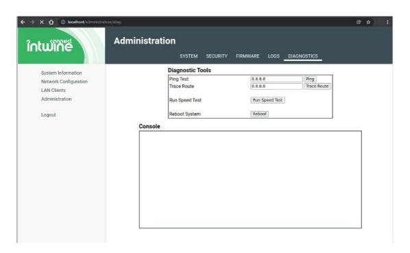
The Diagnostics tab allows users to conduct tests to help determine that their system is properly working or to isolate and resolve problems. Users can make the ICG-200 ping a specific IP address or URL as well as run a traceroute. These tests can allow you to resolve network connectivity problems. Users can also have the system run a speed test and
