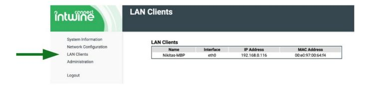
The LAN Clients tab shows a complete listing of all WiFi and/or Ethernet devices that are connected to the gateway. Each LAN client will show its Interface (WiFi/Ethernet), IP Address, and MAC Address, and for devices that have been assigned a Name, that will show as well.
