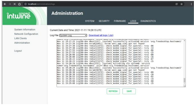
The Logs tab allows users to take a look at or download the logs. The available log files are — **System Log**, **Application Framework**, **Network Config daemon**, **and ICG Log**.
