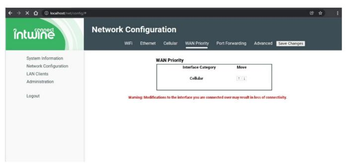
Allows users to choose primary and secondary WAN connections. For example, in a typical cellular backup scenario, a user will want to configure Ethernet as the Primary WAN (priority 1) and Cellular as the backup WAN (priority 2), in case of a network outage.
