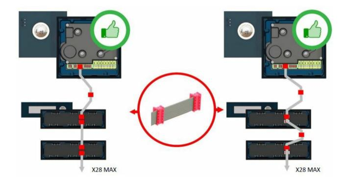
• For lengths over 25 cm, you can use additional cables ref 32-1001. Cut the flat cable to the desired length. It is not necessary to connect all the connectors.
