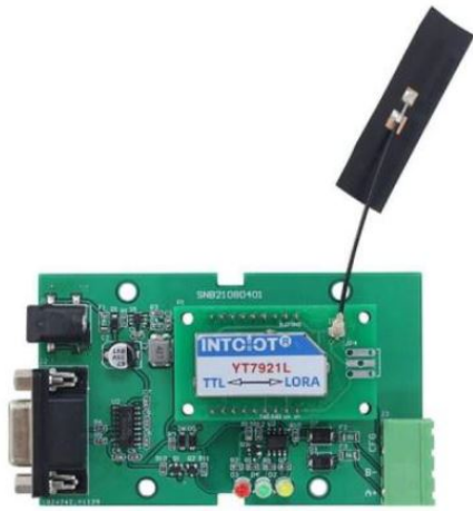
Real shot photos of LoRa module with test board
