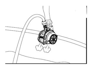
**CAUTION:** Do not pull the hose directly which could damage the auto cleaner hose connection fitting.
