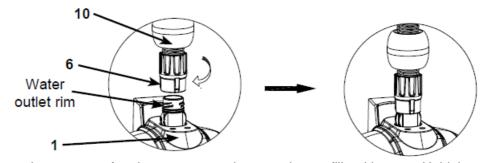
5. Venting the system is necessary for air to escape as the auto cleaner fills with water. Hold the auto cleaner handle and slowly lower it into the pool water. Hold the hose vertically and slowly submerge the hose into the water section by section to remove all the trapped air in the hose. Stretch out the hose by slowly pulling the auto cleaner across the pool to the opposite side. Make sure the hose is stretched out in order to prevent any entanglement. See Fig. 5.
