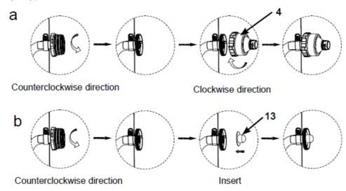
**NOTE:** When cleaning is completed, make sure to remove the hose adaptor (4) and the suction outlet plug (13), and replace the strainer grids back to the water outlet connectors.
