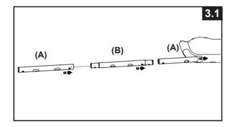
Keep the metal beam holes aligned with the white liner sleeve holes. Continue inserting all "A-B-A" beams into the sleeve openings.
