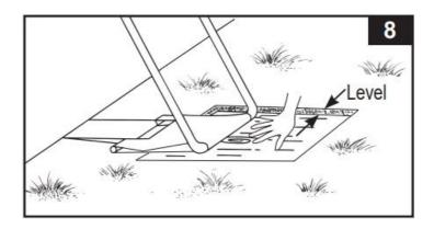
**NOTE:** Make sure each support pad is recessed and set flush with the ground and not just placed on the ground. Do not use support pads or slabs with slippery, smooth surfaces as the U-shaped side support will slide outward causing damage to the pool and void the warranty.
