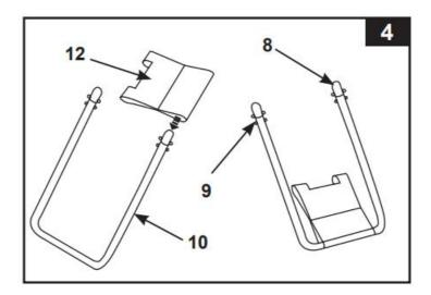
5. The tops of the U-shaped side supports have a double button spring loaded clip (9) that is factory pre-installed. Insert the side supports into the "A-B-A & D" beam holes by squeezing the bottom button inward with your fingers. Squeezing this bottom button will allow the support to enter the beam. Once the U-support is inside the beam release the finger pressure allowing the support to "SNAP" into place. Repeat this procedure for all U-shaped side supports (see drawing 5).
