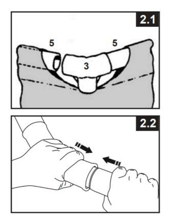
The last joint connection may be difficult to complete. You can do it though, if you first simultaneously raise the last joint and beam about 2 inches (5cm). Now insert the beam into the joint while lowering the pieces into position. The beam will easily slide into the joint (see drawing 2.3). Ensure that the last joint is fully connected before proceeding to connecting the legs.
