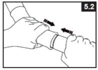
• The last joint connection may be difficult to complete. You can do it though if you first simultaneously raise the last joint and beam about 2 inches (5cm). Now, insert the beam into the joint while lowering the pieces into position. The beam will easily slide into the joint (see drawing 5.3). Ensure that the last joint is fully connected before proceeding to connect the legs.
