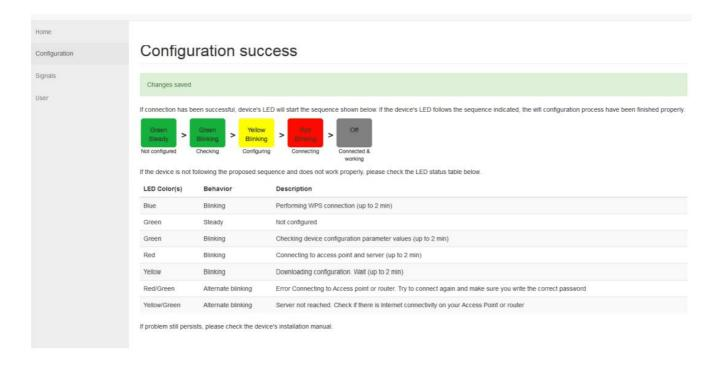
If process does not finish properly (LED is not OFF), the configuration process failed in some point (for example, wrong password used or others).
