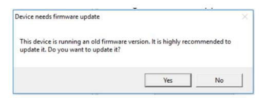
During the firmware update, the device might disappear from the list or the name might change into red. Once the process finishes, device restarts and after a few seconds will be available in the list.
