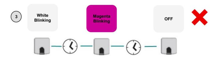
In this case, connect the device to a local WiFi network with accessible Internet connection or check the quality of the Internet signal.
