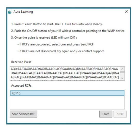
Finally, once the correct RCF is selected from the list, press **Send Selected RCF** and automatically **Subfamily** and **Model** will be filled according to your remote.
