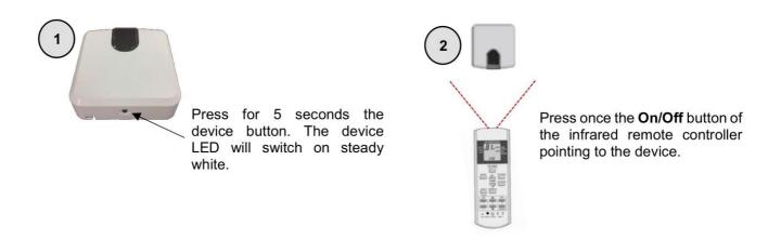
After pressing the ON/OFF button towards the INWMPUNI001I000 device, there are different sequences that can result from this process:
