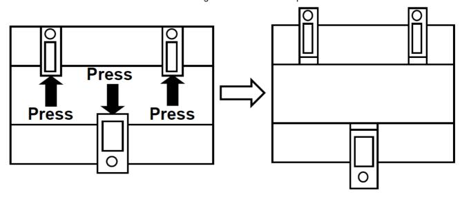
With the clips of the box in their original position, insert first the box in the upper edge of the DIN rail and later insert the box in the down part of the rail, using a small screwdriver and following the steps in the figure below.
