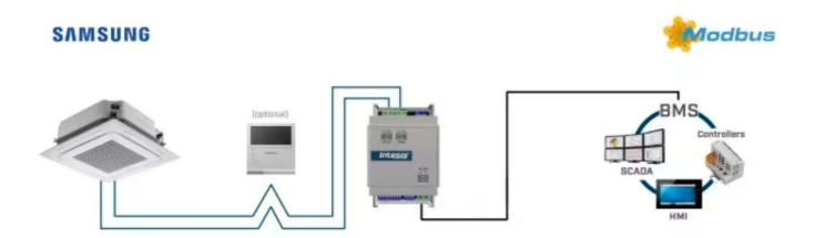
Samsung to Modbus RTU - 1 indoor unit
