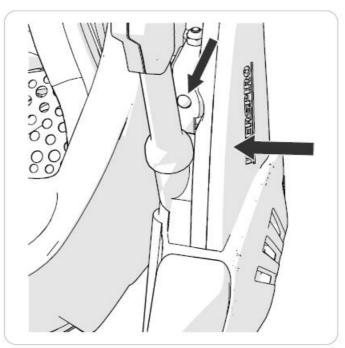
3. Hand screw version: Press the Spirocom against the mask until it is possible to tighten the hand screw moderately in the hole in the attachment bracket.
