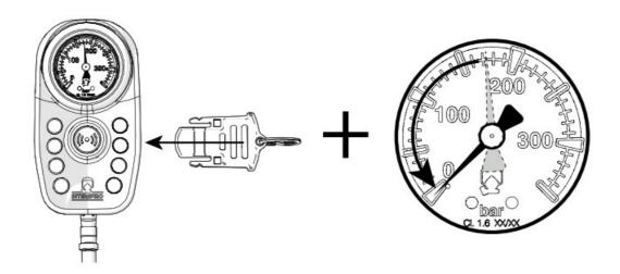
Depressurize the SCBA to 0 bar and then press the mode button and alarm button at the same time.
