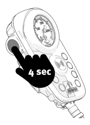
The battery status can only be checked when the unit is off. When the PAC is on it will make an alarm when the battery level drops below 2 hours of usage.
