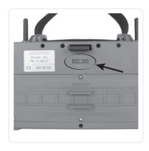
2. Battery status and network indication are alternately displayed on the LED; with long pulses (battery) and shorter pulses (network).
