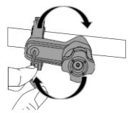
Insert, push and rotate 45 degrees to lock
