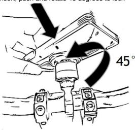
Push and rotate 45 degrees to unlock
