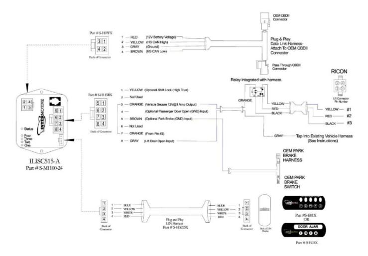
If the ILISC515-A fails any step in the Post Installation Test, review the installation instructions and check all connections. If necessary, call InterMotive Technical Support at <u>530-823-1048</u>.
