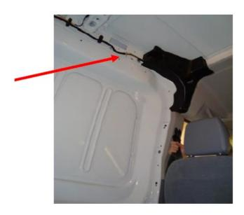
If a "Key OFF" operation is desired, a discrete Lift Door input must be made to the module. This is accomplished by connecting to the existing vehicle switch harness above and behind the driver's seat. Securely connect the Gray wire of the 8-pin harness to the Yellow OEM wire. If using a Posi-Tap, follow the below instructions.
