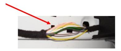
Unscrew the other end of the Posi-Tap connector, strip 1/4" insulation off the Gray wire coming from pin 8 of the module, and insert it through the loose piece so the wire end is even with the piece edge. Hold the wire so it doesn't push back out of the Posi-tap, and screw it back into the main Posi-Tap body. Holding the main Posi-Tap body, gently pull on the just-installed wire to make sure it is solidly connected. Secure the connection using tape.
