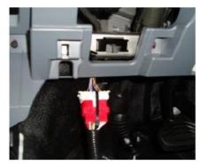
5. Plug the free end of the Data Link harness into the mating 4-pin connector on the ILISC515-A module.
