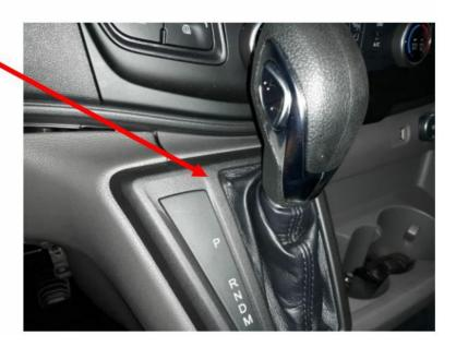
Remove the two screws shown in the photo.
