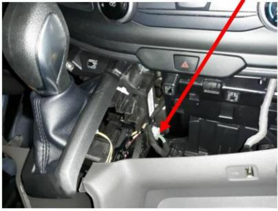
Locate connector 2810 (12-pin connector). Remove the OEM connector and plug it into the mating 12-pin connector T-harness. Plug the male connector into the OEM mating connector.
