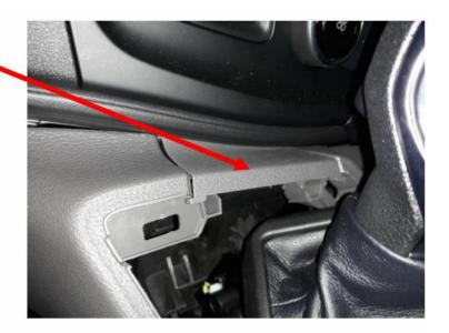
Remove the center dash panel by pulling it towards the rear of the vehicle.
