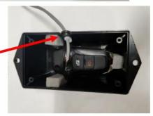
Replace the cover onto the box and secure it with the 4 included screws. Plug the 3-pin connector into the mating connector on the key fob harness.
