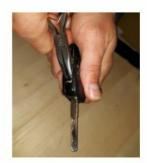
5. Remove the switchblade key, the battery, and the silver loop from the back (optional).
