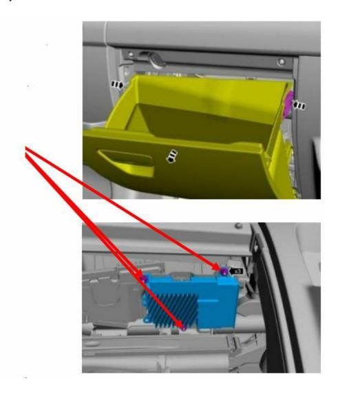
1. Locate the vehicle's Gateway Module. It will be mounted behind the glove compartment.
