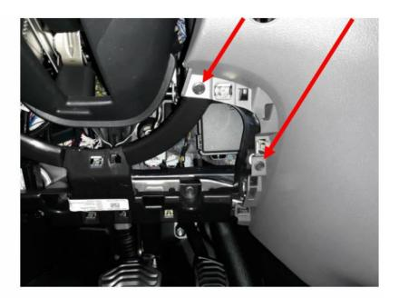
Remove the trim panel on the passenger side by using a plastic trim removal tool.
