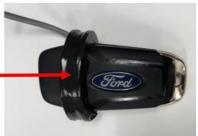
Insert the key fob into the bottom of the key fob box and route the harness toward the hole on the side of the box. Place the rubber grommet in the hole as shown.
