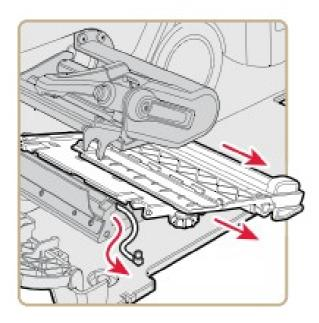
6. Insert the RFID antenna into the media guide assembly.
