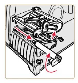
3. Use the T10 Torx screwdriver to remove the three screws that secure the plate on the outside of the media guide assembly.
