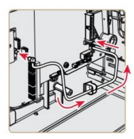
6. Insert the RFID ribbon cable into the 80-pin connector on the printer main board.
