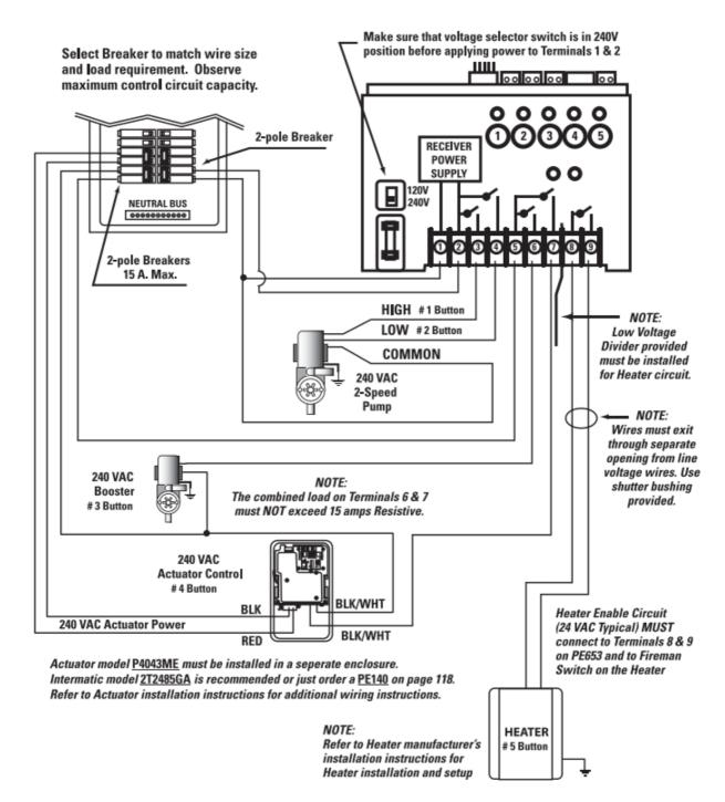
240 V 2-Speed Pump + 240 V Blower + 240 V Actuator +Heater
