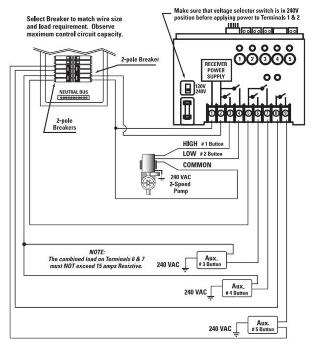
240 V 2-Speed Pump + Booster Pump + 120 V Light +Heater
