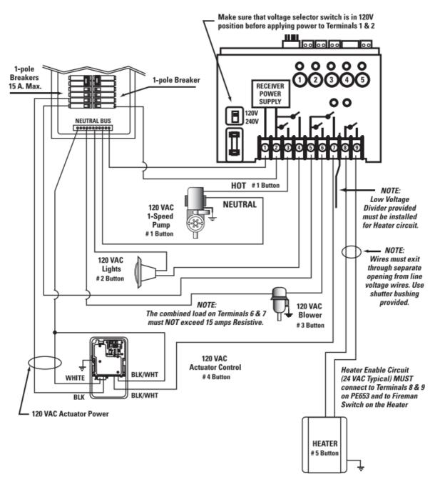
Actuator model P4843ME must be installed in a separate enclosure. Intermatic model 2T2485GA is recommended or just order a PF14Q on page 118. Refer to Actuator installation instructions for additional wiring instructions.
