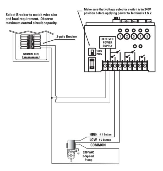
240 V 2-Speed Pump + 240 V Booster Pump + other 120 VAC Equipment + Heater
